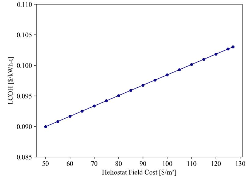
Sensitivity analysis for heliostat field cost. Maximum is the current SAM cost, while minimum is the DOE target heliostat cost.
