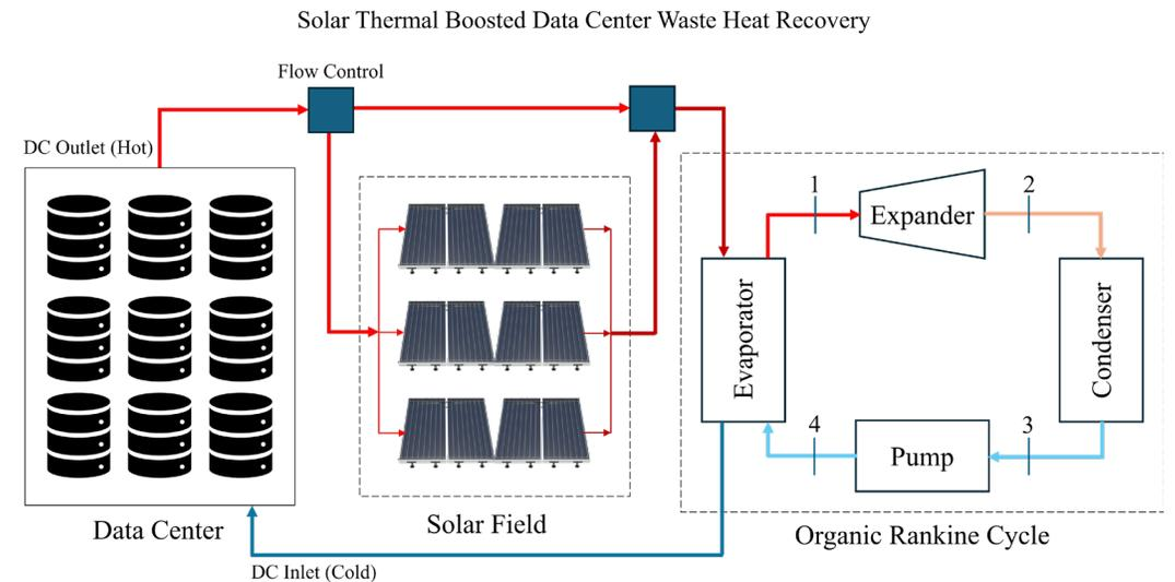
Solar thermal boosted WHR system for data centers
