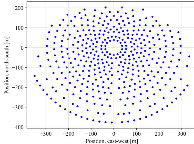
Thermal storage and solar field sizing (left), SolarPILOT optimized solar field layout (right)
