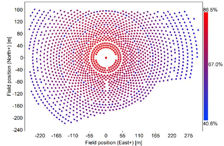
SolarPILOT optimized heliostat field for MSPT
