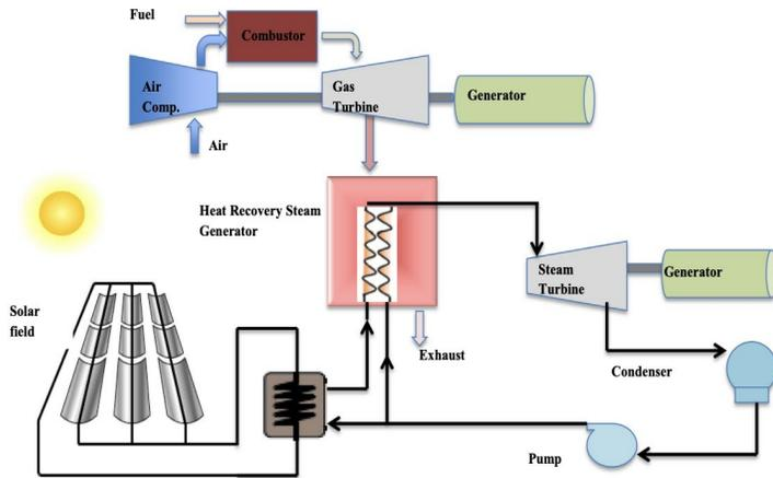
Fig. 1. Diagram of an ISCC plant.
