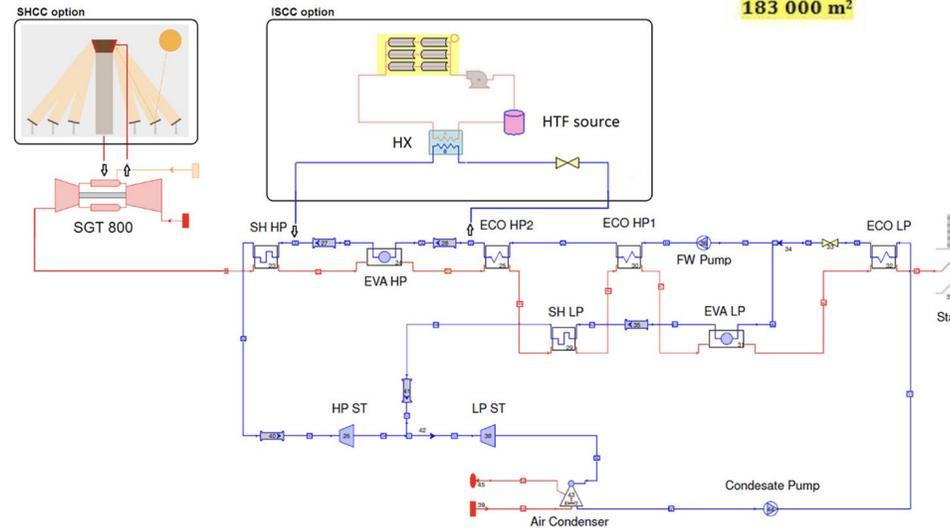
Fig. 1 Schematic of the investigated solar-fossil combined cycle: ISCC versus SHCC option
