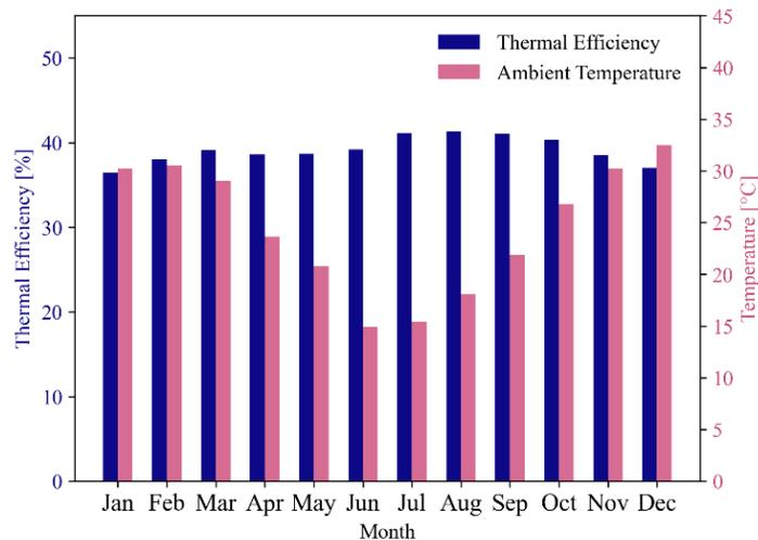
Monthly power cycle efficiency and ambient temperature
