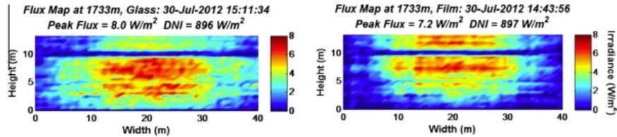
Fig. 9. Measured irradiance distribution at ~1700 m from the silvered glass facet (left) and the SMF1100 facet (right). The peak flux in both cases is ~7–8 W/m<sup>2</sup>.
