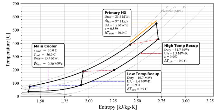
T-S diagram for sCO<sub>2</sub> cycle, simple (top), recompression (bottom)
