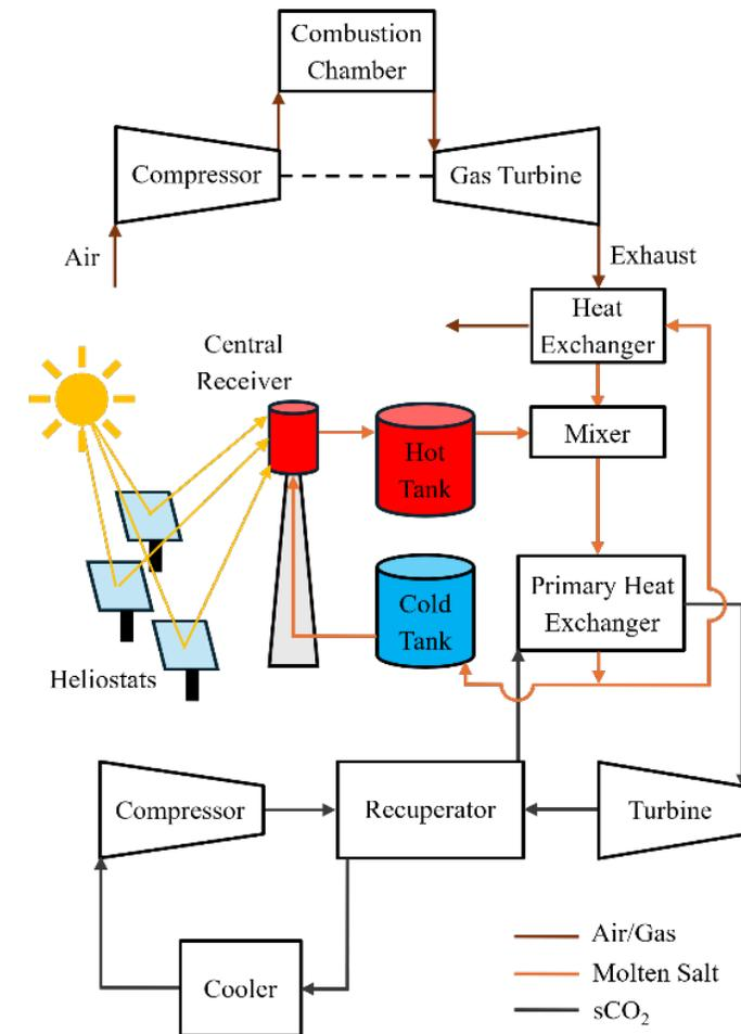
Schematics of the proposed CSP-sCO<sub>2</sub> hybrid WHR system
