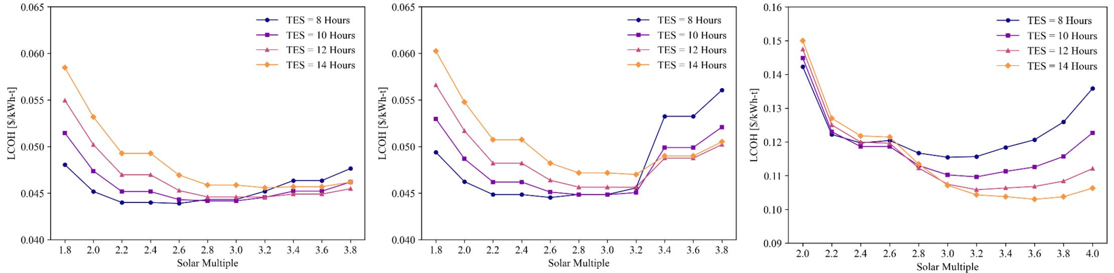
Parametric optimization of solar field (SM) and TES sizing. PTC-150°C (left), PTC-300°C (center), and MSPT-574°C (right).
