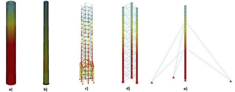
FIGURE 3. FE-models of investigated tower designs: a) concrete tube, diameter 22 m; b) concrete tube, diameter 15 m; c) lattice steel tower with socket; d) three-leg hybrid tower with concrete columns and steel bracings; e) cable-stayed concrete tube with two layers of cables
